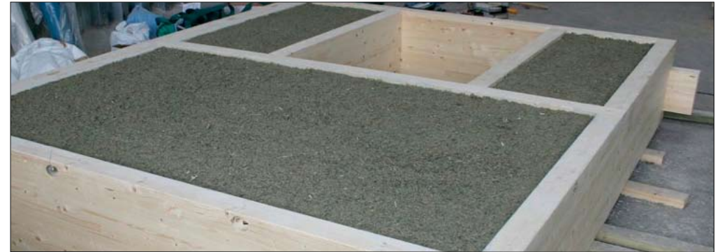
A timber framed, straw bale panel in manufacture
